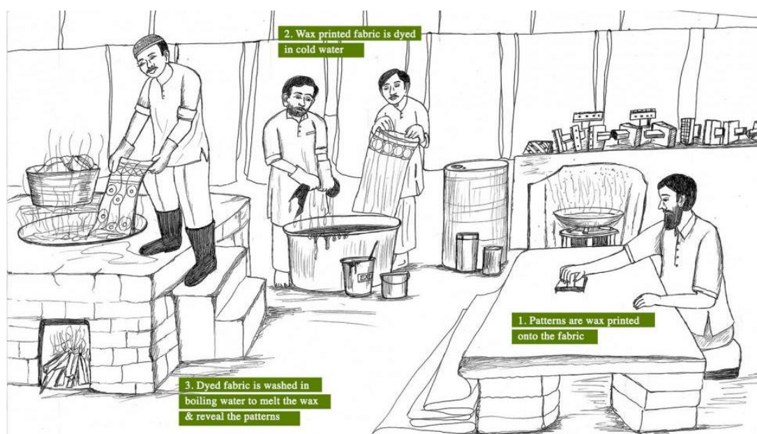
3.2.8 Illustrative depiction of the process of batik printing on fabric
