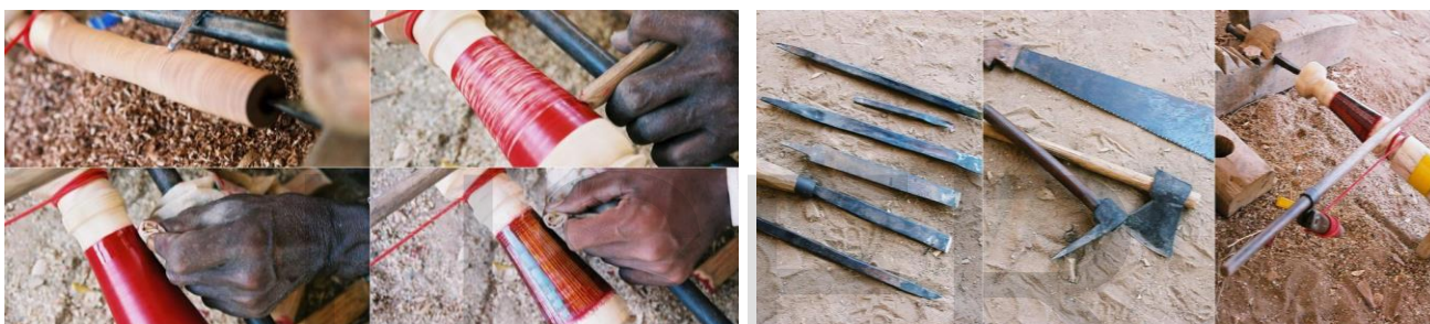
3.2.12 Tools and process involved in lacquered woodwork documented by Khamir, Kutch
