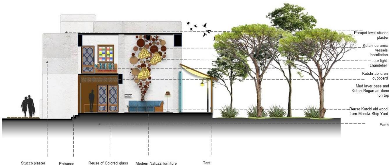
4.2 Schematic section highlighting the design approach
